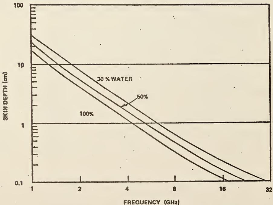
Figure A-4 Skindepth vs Frequency for Water (100% Curve) and for Media whose Dielectric Constant is 50 and 30% respectively of the Dielectric Constant of Water (Aerojet-General Independent Research)
